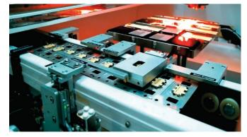
Figure 2: "Universal" progress indexing conveyor.
