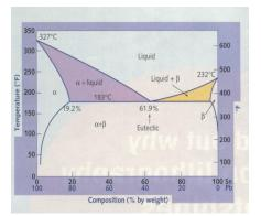
**Figure 1:** Eutectic transitions for a given metal composition—in this case, tin-lead.
