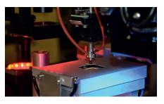
Figure 2: A pulse-heated, fast-ramp eutectic stage.
